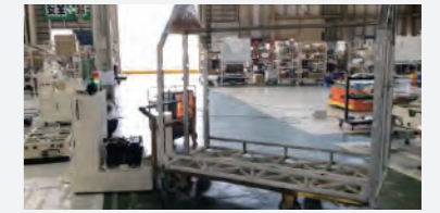
Quick reverse for automatic coupling between a platform and pins.
